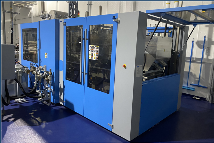
(2017) SIPA Linear blowmoulder machine Model: SFL1XL
