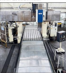
TOSHIBA SHIBAURA MPE-2140 CNC 5 FACE GANTRY MILL
